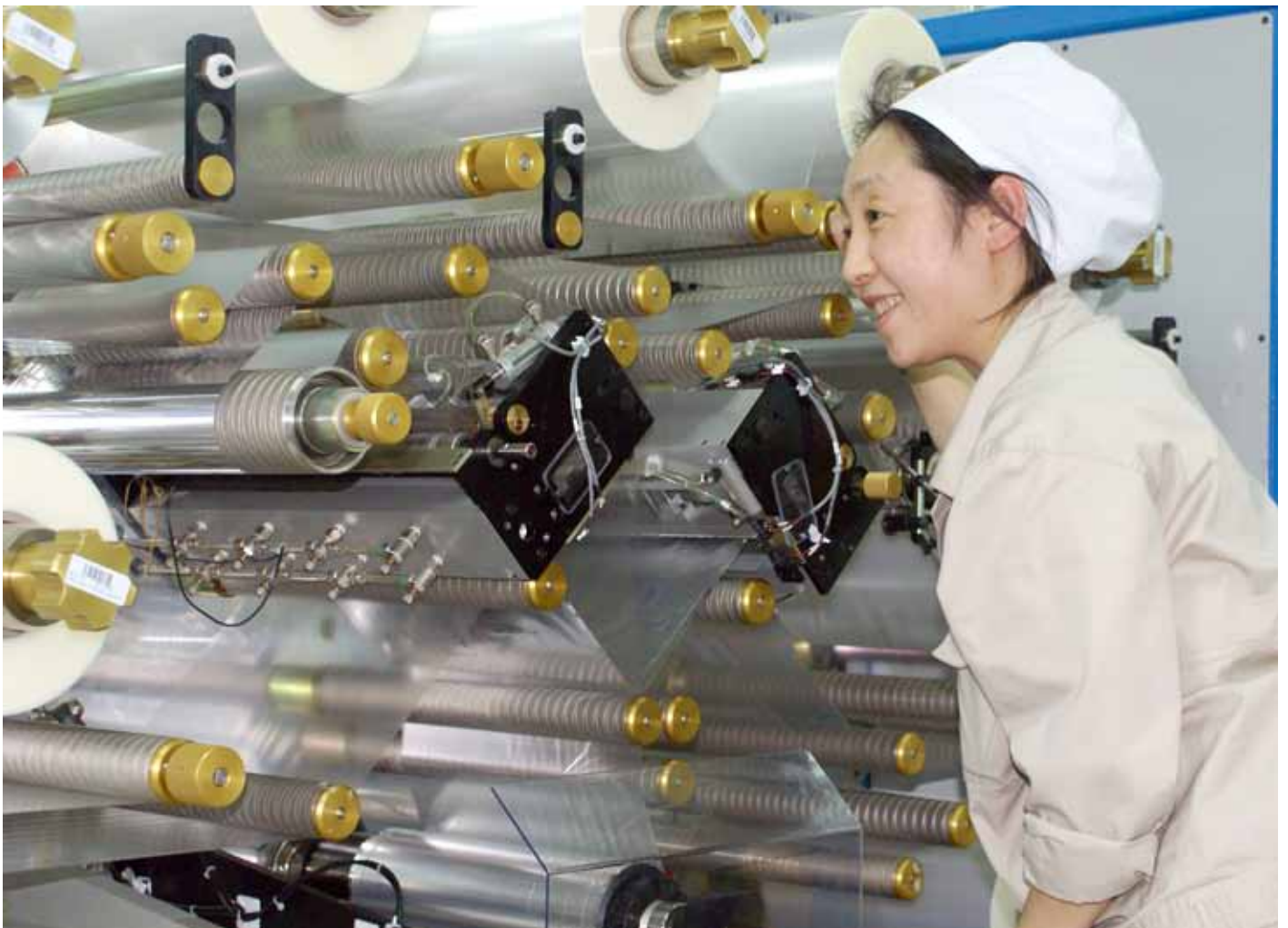
Process inspection of element winding
